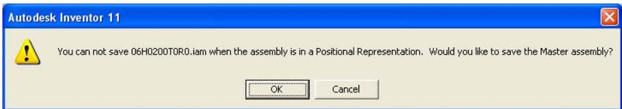
**Figure 3 - Saving the assembly in a non-master ViewRep**
